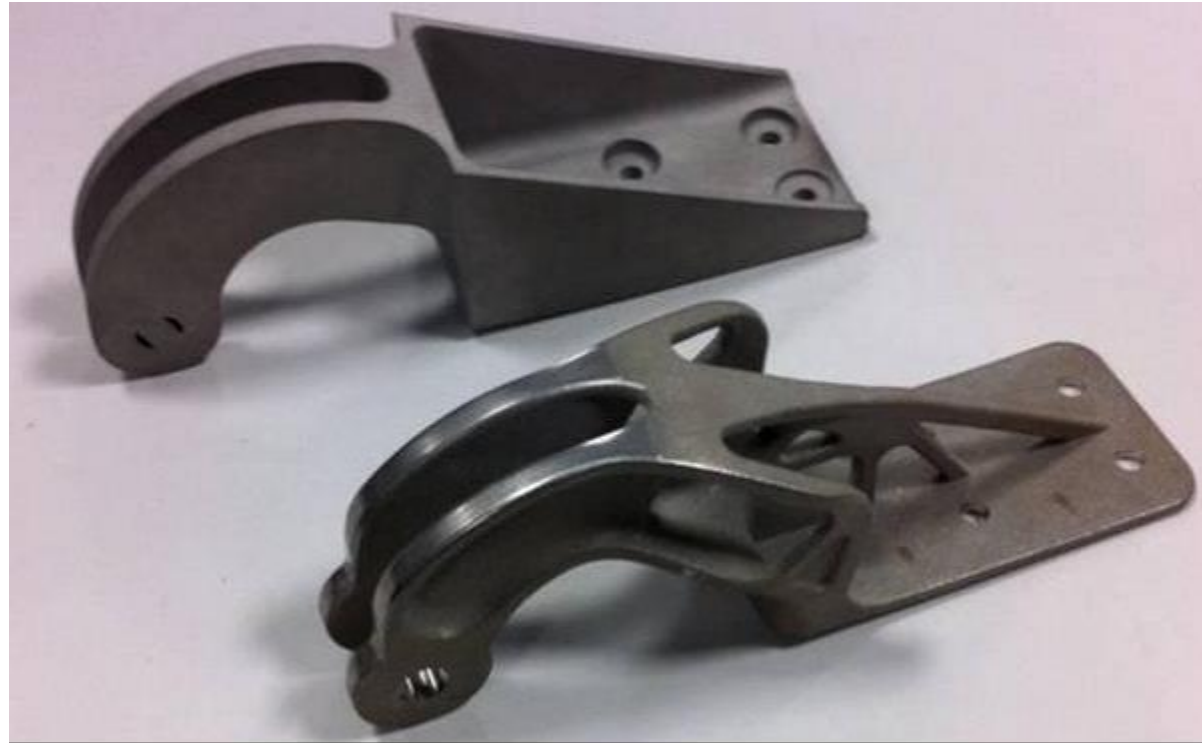
Hinges for the Airbus A320 - conventional (background) and 3D printed (foreground)
